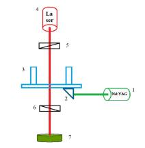
Fig. 1. Scheme of the experimental setup. 1 – Nd: YAG quasi-continuous laser; 2 – prism; 3 – cell; 4 – probe laser; 5, 6 – polarizers; 7 – power meter.
