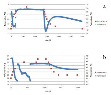
Fig. 2. Dependence of temperature and transmittance coefficient of probe beam on time. In a) and b) cases the directions of hydrodynamic flows are opposed to each other.
