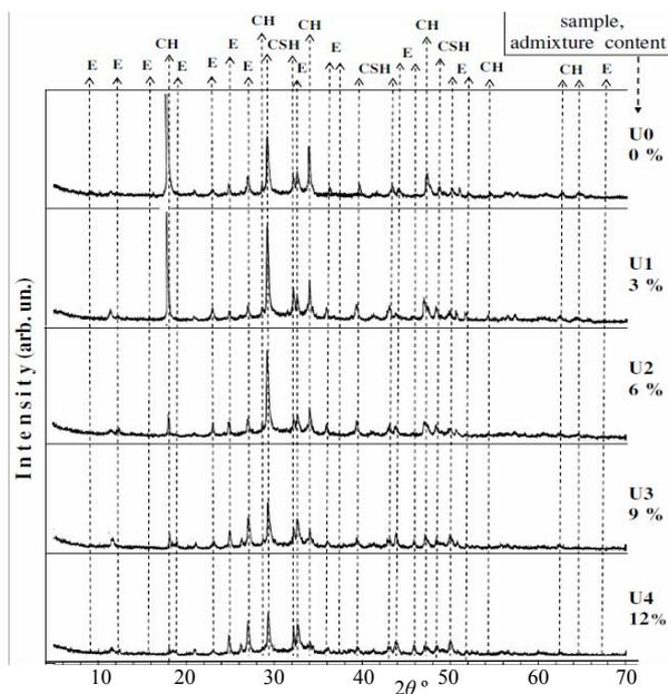
Fig. 1. The  $\text{CuK}\alpha$  XRD spectra recorded from cement paste samples. Identified diffraction peaks belong to main hydration phases: ettringite (E), calcium hydroxide (CH), and calcium-silicate-hydrate (CSH).
