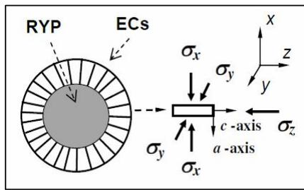
Fig. 2. Modeled “ye’elinite-ettringite” cluster composed of a residual ye’elinite particle (RYP) and a shell of ettringite crystals (ECs).
