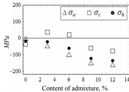
Fig. 3. Dependence of the stress components on ettringite crystals on the relative content of ye’elinite admixture.
